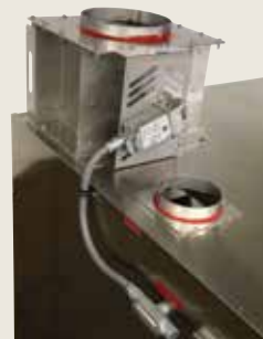
Smoke Extractor installed on the smoker and wired into the existing wire hub
